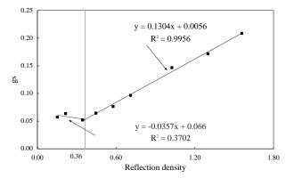
Figure 3. The gs for graininess JND patches plotted versus the mean reflection density and two regression lines.
