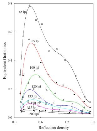
Figure 6. Equivalent graininess applied to all the patches on Test Chart No. 4.
