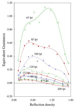
Figure A. Equivalent graininess (by Model 1) applied to all the patches on Test Chart No.4.
