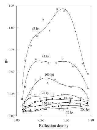
Figure 2. The gs of each patch plotted versus the mean reflection density according to each screen ruling.
