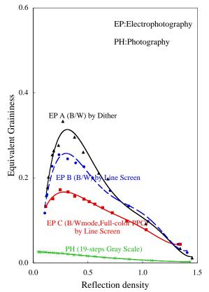
Figure B. Equivalent graininess (by conventional metric) applied to gray-scale images by electrophotography and photography.
